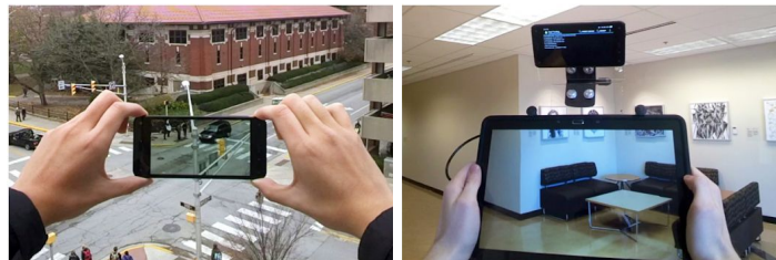
Video-see-through AR displays: simulated transparency
